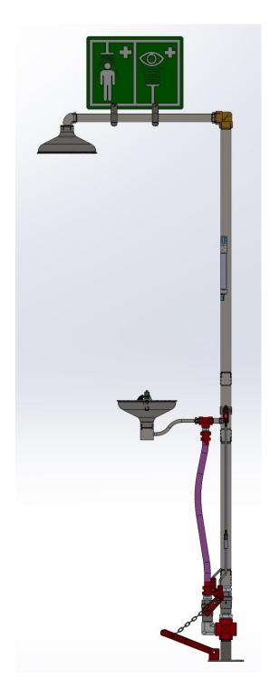
Designed for hot climates. The power of the sun can heat standing water within the pipes of an emergency safety shower to temperatures as high as 50°C. The self-draining valve releases potentially scalding water from the standpipe to avoid further shock or injury to the casualty. Meets EN15154 and ANSI standards.
